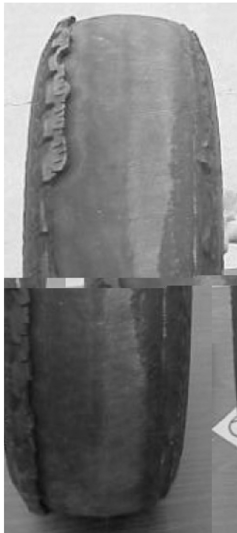
FIG. 2. — Tire carcass after a complete tread separation. (reprinted from Ref. 1 – the NHTSA ODI report EA 23).
